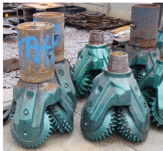
LDD drill bits used during drilling at KX36.
